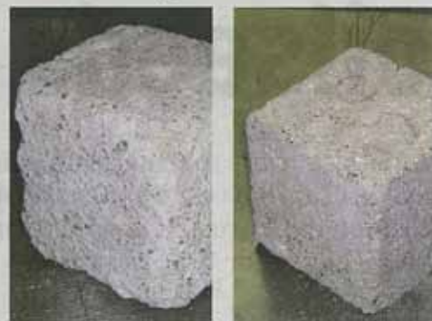
LEFT: Concrete made with 100% Portland Cement RIGHT: Concrete made with 50% GGBS cement and 50% Portland cement.
